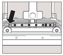
Unscrew the track with an AWK (allen wrench) and remove it from the retainer.
